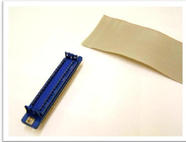
**Figure 7:** The ribbon cable removed from the connector.
