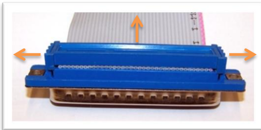
Figure 5: Gently pull side retainers away from the connector to release the connector backing
