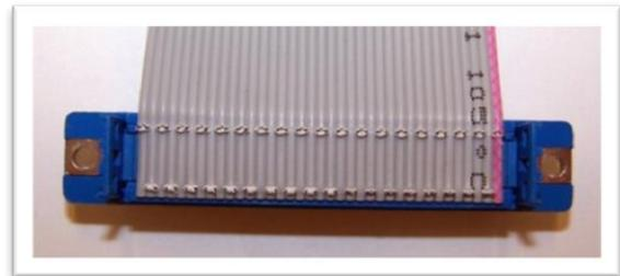
Figure 6: The connector with the connector backing removed.
