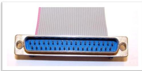
Figure 3: The male end of the cable assembly
